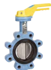
1181 - Disc CF8M up to DN100, Disc GGG50 epoxy coated above / Seat NBR For gas - PS: 5 bar (class MOP5) - TS: -20°C/+60°C.
