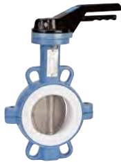
1145 - Disc CF8M / Seat Teflon® with silicone liner TS: -25°C/+200°C.
