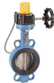
1144 - Disc CF8M up to DN100, Disc GGG50 epoxy coated above / Seat EPDM For fire network - FM approved - With gearbox & limit switches - TS: -10°C/+110°C.
