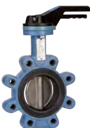
1163 - Disc CF8M / Seat EPDM TS: -10°C/+110°C.
