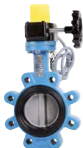
1182 - Disc CF8M up to DN100, Disc GGG50 epoxy coated above / Seat EPDM For fire network - FM approved - With gearbox & limit switches - TS: -10°C/+110°C.
