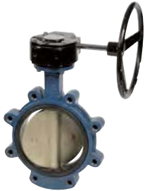
1135 - Gearbox - Disc GGG40 nickel plated / Seat EPDM
